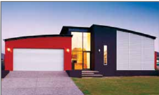
FIGURE 6: Example of curved roof house with a radius not greater than 40m and with two distinct sections (Source: WA Country Builders, 2009)
